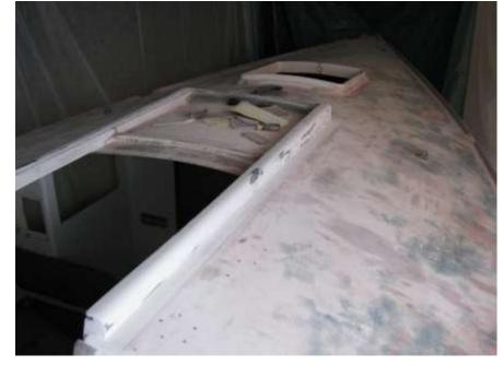
Spraying the deck made a big difference to the appearance of the boat, no longer was the deck covered in holes from previous fittings. We applied some non-slip granulues into the last layer of paint being sprayed on to give some much needed grip.
