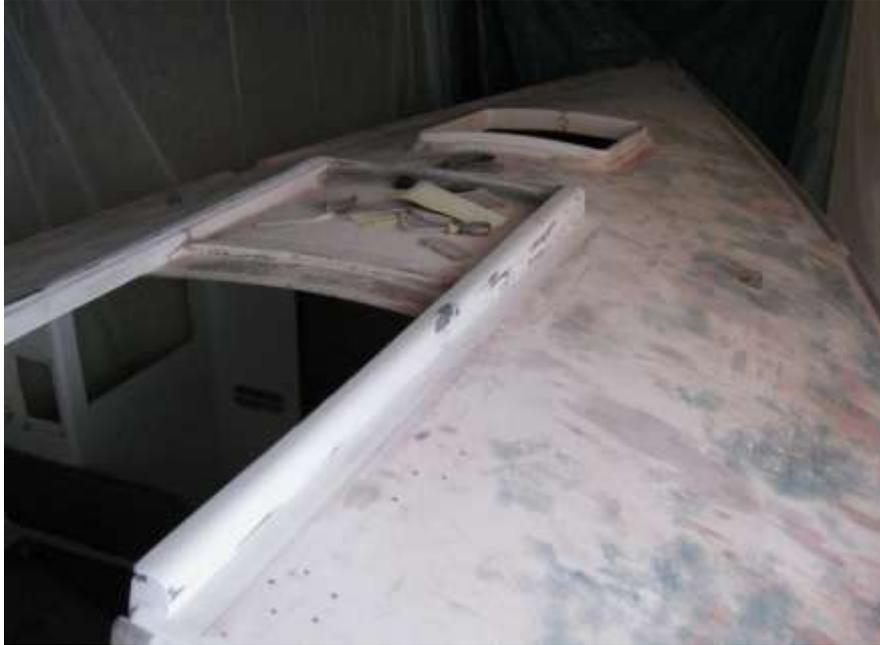
Spraying the deck made a big difference to the appearance of the boat, no longer was the deck covered in holes from previous fittings. We applied some non-slip granules into the last layer of paint being sprayed on to give some much needed grip.
